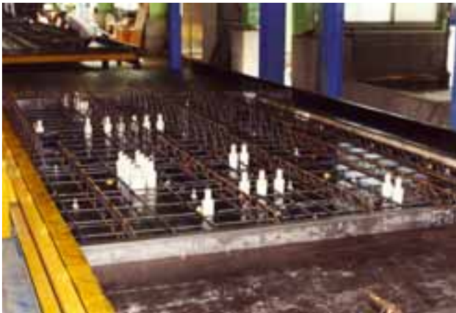
Reinforced pallet with recess bodies and threaded sockets
