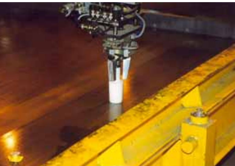
The insert robot positions a recess body
