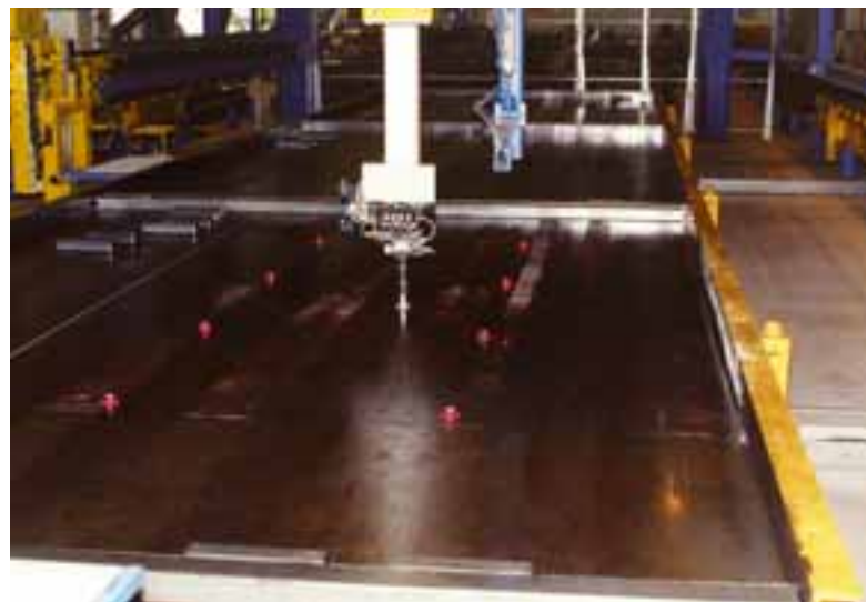
The insert robot positions threaded sockets
