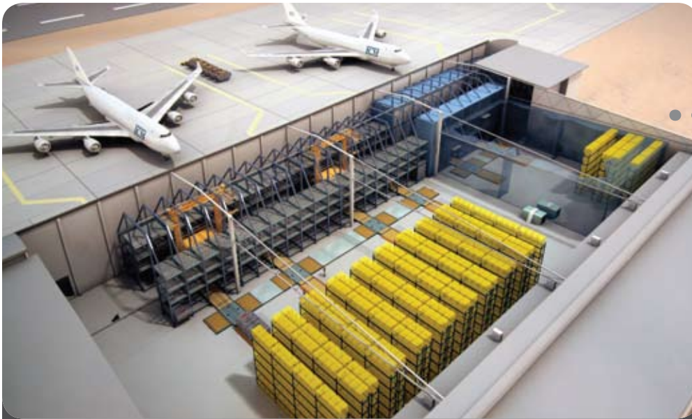
A 3-D graphical representation of the cargo handling system showing the roller decks, the ETV's and the cold storage area
