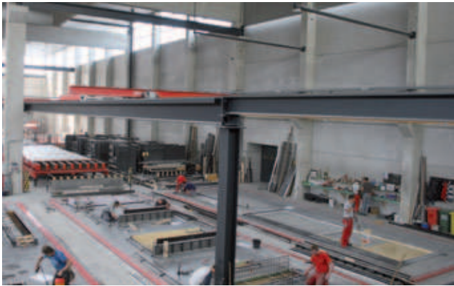
A good view of all stations is provided from the control room. Unitechnik laser projectors are installed centrally above stations M01 and M02
