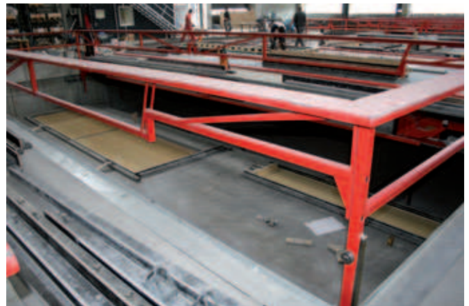
After a workplace has been secured by its guard rail, the elevating platform from the basement level takes hold of the pallet, lowers it and transports it to the next station
