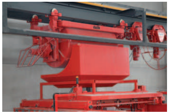
The Dudik bucket conveyor transfers concrete to the concrete spreader
