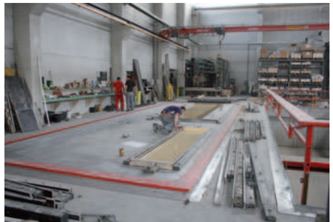
Special components, as manufactured to order by Nägelebau, demand a great deal of manual activity in setting up the formwork
