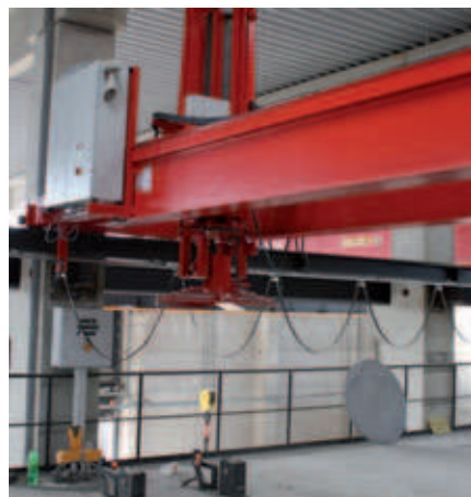
Power trowel above the curing chamber
