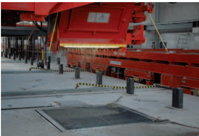
Integrated cleaning station immediately adjacent to the concreting station
