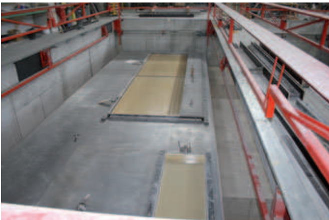
After a workplace has been secured by its guard rail, the elevating platform from the basement level takes hold of the pallet, lowers it and transports it to the next station
