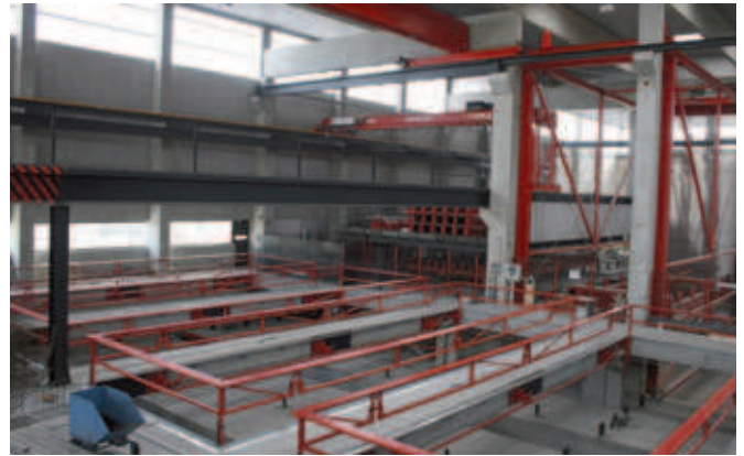
A good view of all stations is provided from the control room. Unitechnik laser projectors are installed centrally above stations M01 and M02
