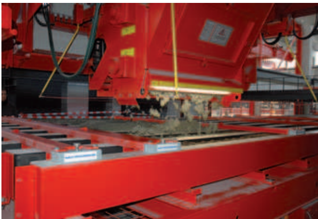
The concrete spreader ensures that the formwork is filled precisely
