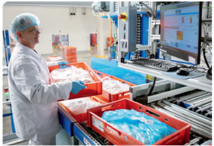
At the workstations, order pickers place the items onto automatically supplied pallets, following instructions provided by the UniWare warehouse management system. Photo: Unitechnik
