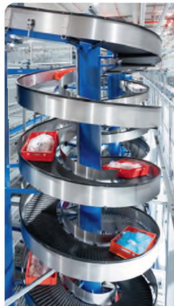
When a customer order is triggered, the required trays are retrieved in the precise sequence needed, removed from the trays and transported via spiral conveyors to the workstations below. Photo: Unitechnik
